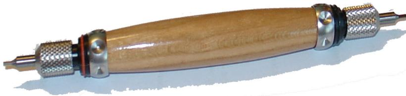
The main applications for this rapid check are internal shapes such as hexagon sockets, rounded toothings, threads, cylinders and also non-circular shapes (!).
